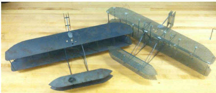
Both 18" wind tunnel models - solid wing and perforated wing - used in UD wind tunnel test project
