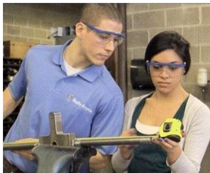
Aero students Hendrickson and Crump measure load cell mounting arm to match wind tunnel specifications
