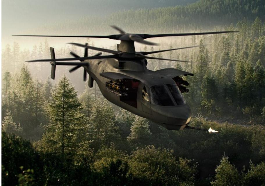
An artist's concept of Sikorsky's Raider X, a candidate for the US Army's Future Attack Reconnaissance Aircraft (FARA). The Army calls it a "knife fighter" on the battlefield of the future. Sikorsky's X2 technology, proven in flight, includes rigid, counter-rotating blades, fly-by-wire flight controls, and an integrated auxiliary propulsion system that will push the aircraft at 250 knots! Raider X is one of 5 designs in competition. The field will down-select to two for a "fly off" in 2023.
